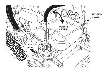
Figure 4-7. Adjusting Steering Levers
